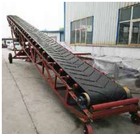
Bag Loading Conveyor
